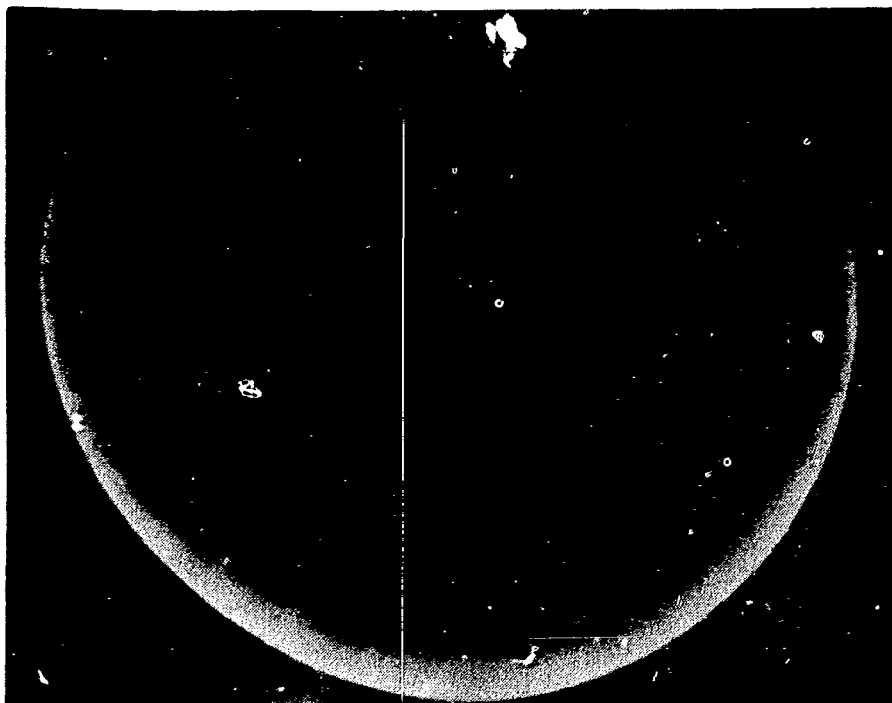
Figure 33. SEM photomicrograph of a typical particle in the upper layer of the Top Region, 22-24" segment, 150x.
